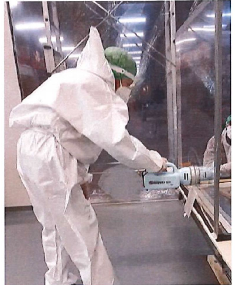
Laboratory test to reduce bacterial load in the Multilevel showcase. Technician during the air sampling phase.
